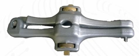
Sheath Stripper, Manufactured by Sunil Co.Ltd is a tool deviced to strip fiber optic cables of sheath with least human efforts. Using Wire Clamp together, you can strip sheath from optical cables more easily and quickly than using knives or handsaws. It's especially convenient when stripping cables for mid span branching. Replacing blades fixed at the center of stripping, you can use this tool pemanently.
